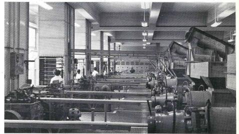
High speed toilet soap making machines (at Mitsuwa's plant)
